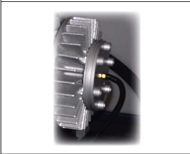
Figure 5-13 High Temperature Switch
